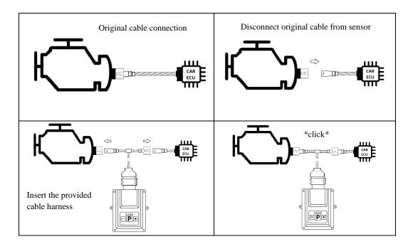
If you need to remove the Tuning Module, please follow the installation preparation procedure; with opening the engine hood, turning the ignition key off, and removing the key from car lock. Afterwards you can disconnect the Tuning Module.
