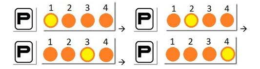
On described drawing the program number 4 - STANDARD is selected, and in order to confirm the selection please wait for 5 seconds that all 4 LED's are finished with flashing.
